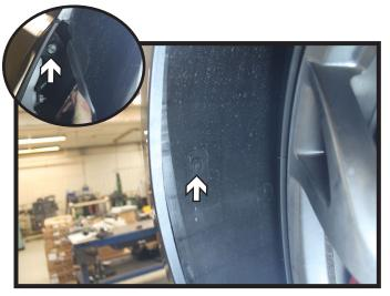
2. Remove the push pin from the wheel well. Pull back the liner and using a 10MM socket, remove the screw the fascia joint (inset).
