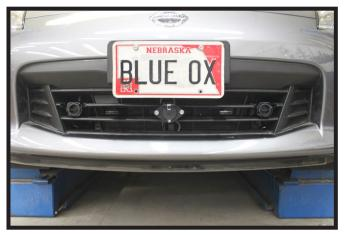
14. Hold the fascia as close to its original position, mark and trim the fascia around the convenience links and attachment tabs. Reinstall the bumper and fascia.
