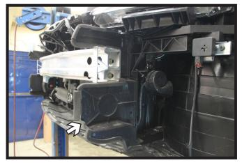
4. Remove the plastic shielding from either side of the bumper. The shields will not be reinstalled.
